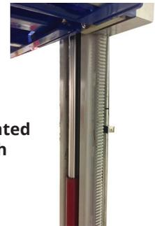
**Rack and pinion style synchronization with cross mounted torsion bar. Push style hydraulic cylinder in each column**
