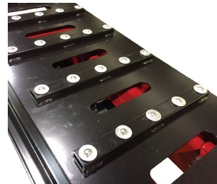
Open runway slots under rear slip plates
