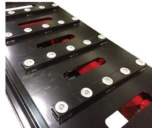
Open runway slots under rear slip plates
