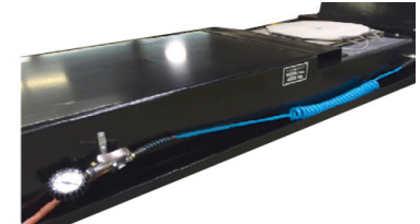
Built in runway tire inflation hoses with pressure gauges #TLSTIL
